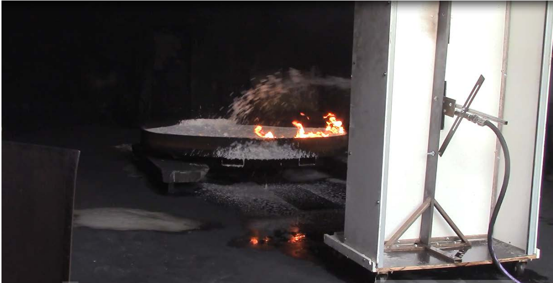
Photograph A3: 90% extinguished test fire
