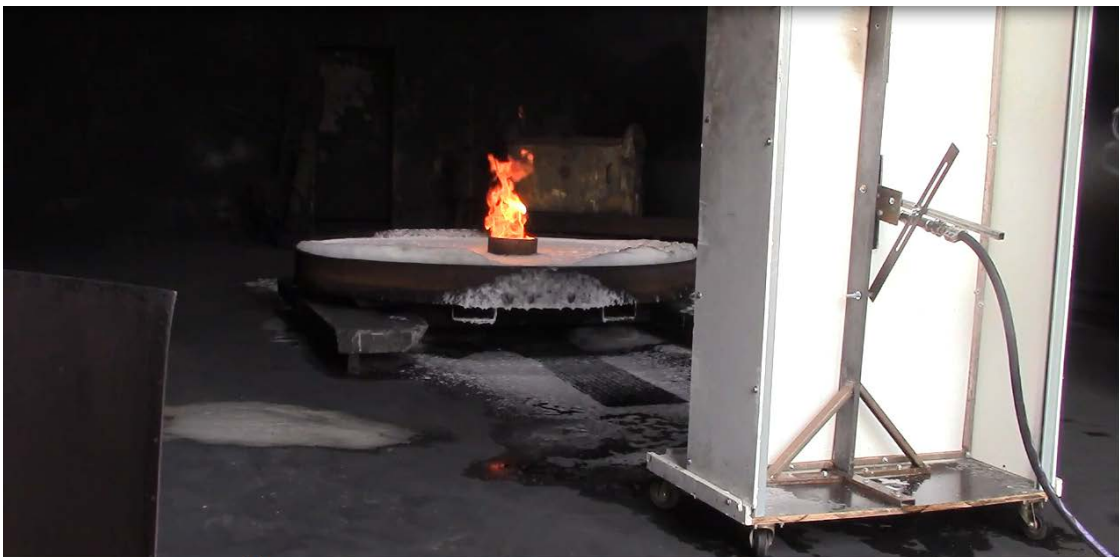
Photograph A4: burn-back test
